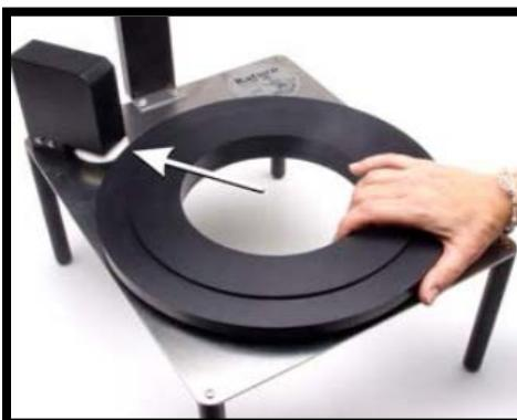
8. Place the Rreturn controller (part F) on a stable, level surface near the base plate (part E). Make sure that both the controller switch (front panel) and the power switch (back panel) of the Rreturn controller are set to OFF. These controls are referenced on page 8 of this manual.
